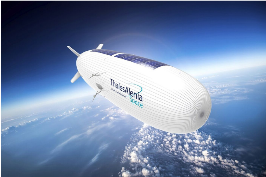
Fig. 11 A depiction of the StratoBus High-Altitude Pseudo-Satellite being developed by Thales Alenia Space for market release in 2021
