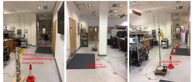
Fig. 4: Measurement setup in the CSN Lab at UoB. A reference measurement is performed without a human body by using the linear rail track and compared to the results with a human body.
