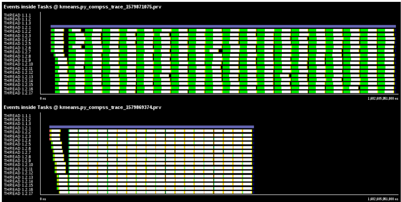
(b) Over the time of the application, reuse of data makes the cost of data serialization insignificant. Parameters are similar to test-case 10.
