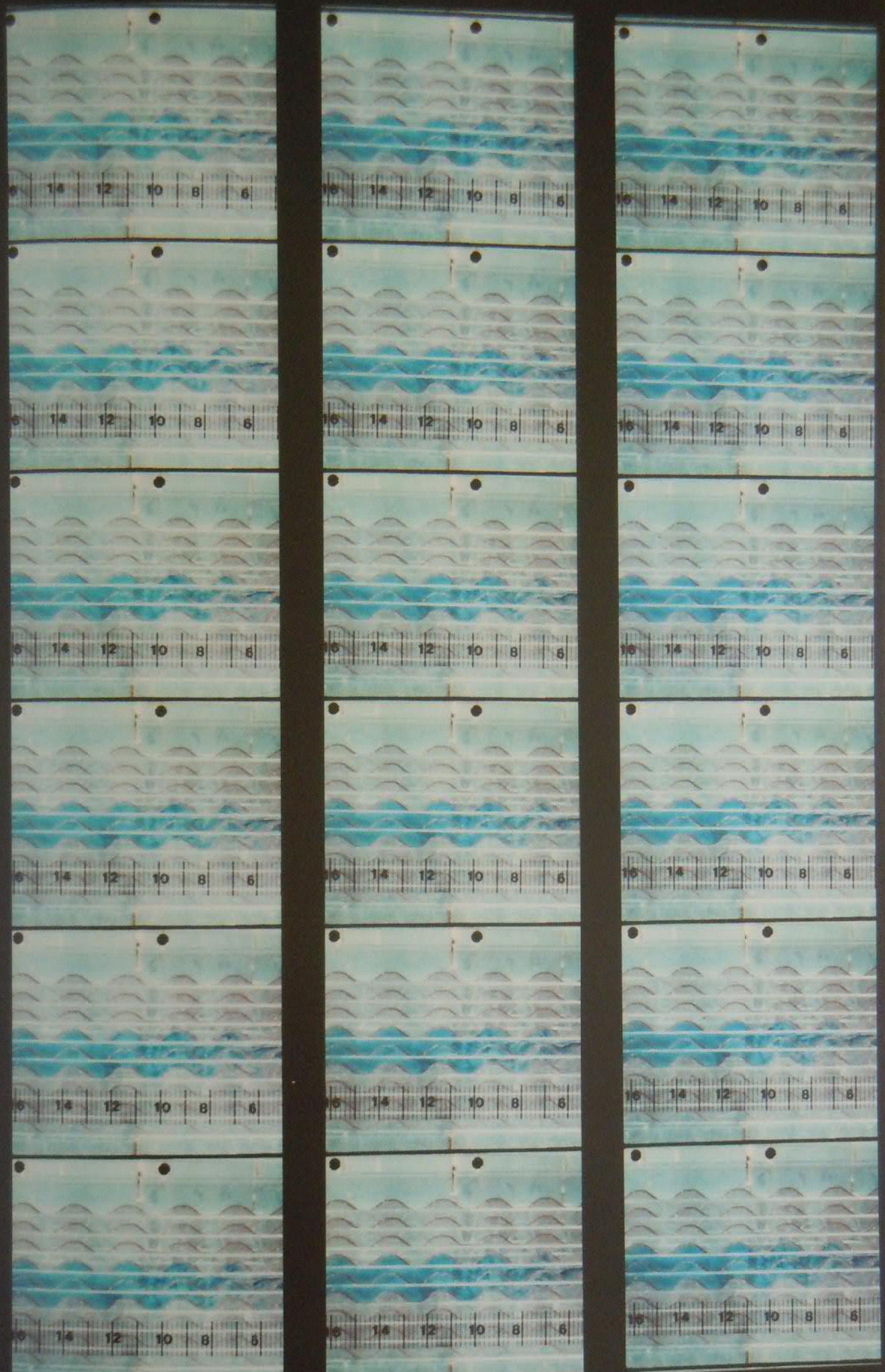
Plate 5.14b Streaklines in duct of profile 3, RH = 0.306 , Re = 1831 wall spacing = 7.25 mm
