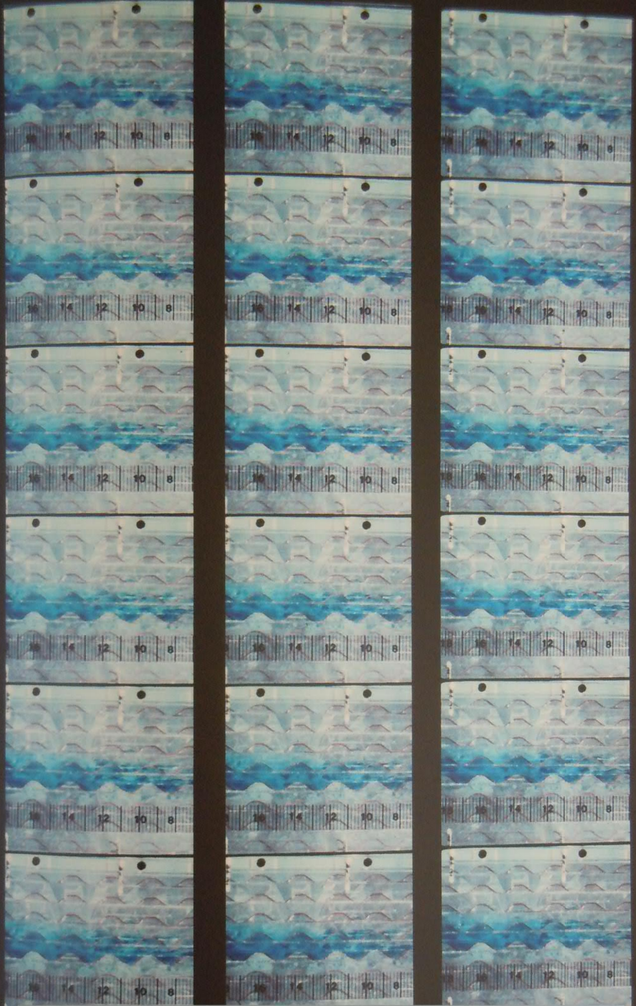
Plate 5.11b Streaklines in duct of profile 3, RH = 0.445 , Re = 1878 wall spacing = 10.55 mm
