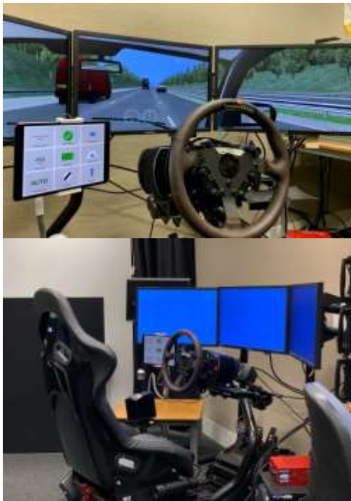
Figure 1 WMG 3xD Development Simulator, with an iPad positioned as a surrogate center console display
