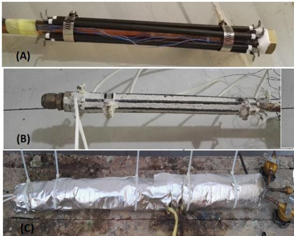
Figure 2. The evaporator heating system: (A) The evaporator section with the heaters. (B) Application of thermal clay between the heaters. (C) Application of thermal insulation glass wool and tape.
