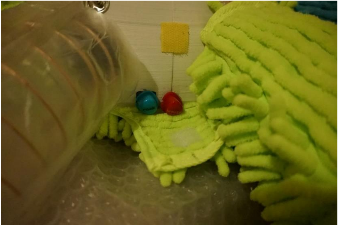
Figure 5.62. Buttons to switch on/off the Raspberry Pi and the LED strips with speakers
