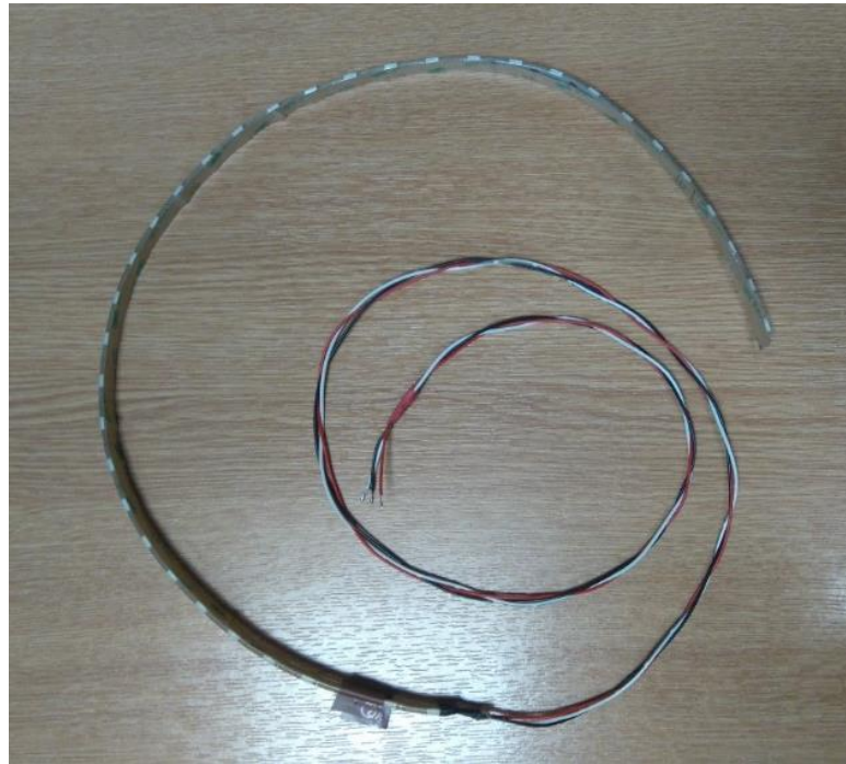
Figure 5.61. LED strip with the extension wire
