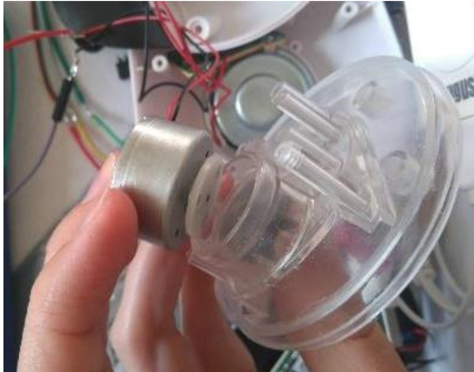
Figure 5.50. DC motor and spiral vessel for fountain speaker
