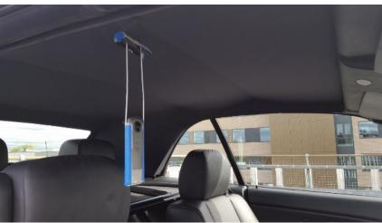
Figure 38. Camera mount rig for Ricoh Theta
