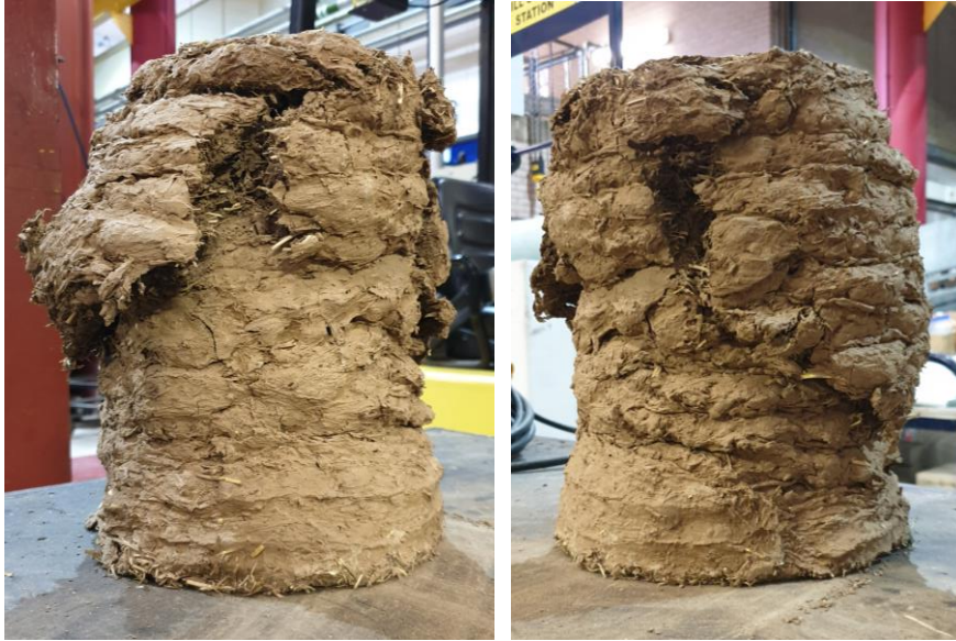
Figure 5: Typical examples of specimens after compressive failure.
