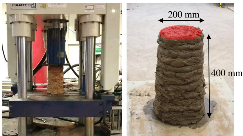
267 268 Figure 4: Compression test setup (left) and the cylindrical specimen (right).
