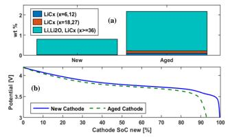
Figure 11 Chemical evaluation of new and aged Li-ion cells showing (a) Nuclear Magnetic Resonance (NMR) results showing increased surface layer formation and (b) cathode half-cell curves for new and aged cells showing noticeable reduction in cathode capacity,
