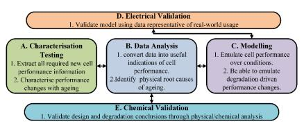
Figure 5 Overall holistic process that incorporates all of the required steps to evaluate ageing in Li-ion cells.
