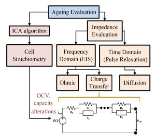
Figure 7 Schematic showing the different aspects of cell behavior that need to be incorporated and the different range of techniques incorporated for quantification including Incremental Capacity Analysis (ICA), Electrochemical Impedance Spectroscopy (EIS) and time domain pulse relaxation. The schematic also shows how each aspect quantifies information for the resultant equivalent circuit.
