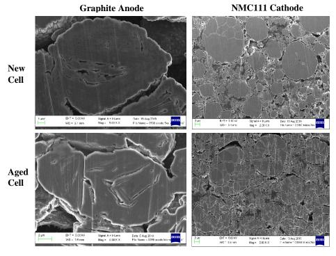
Figure 12 SEM images of anode and cathode samples under identical resolution for the new and both aged cells. All Graphite Anode images are at 5K magnification and NMC111 Cathode images are at 2k. magnification. Images included to show clear deterioration of the cathode and minor deterioration of cathode at the aged cell condition of 9 months of cycling
