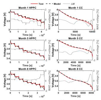
Figure 9 Validation of ageing model against reference test progiles of a hybrid pulse power characterization (HPPC) and a constant current (CC) discharge. Shown at beginning of life (Month 0), Mid-Life (Month 5) and near end of life (Month 8)
