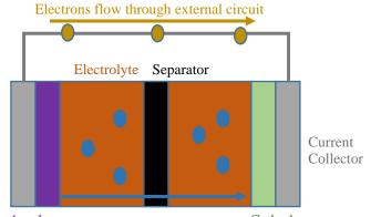
Anode Li-ions flow through electrolyte Cathode
