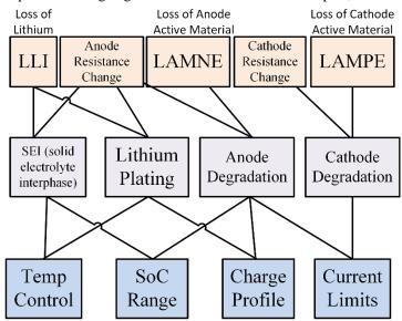
Figure 8 Link between ageing modes, mechanisms, and control aspects. The top row shows types of degradation modes, the middle row their underlying cause, and the bottom row the sensitivities of those mechanisms in terms of controllable usage conditions.
