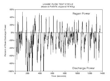
*Figure 6 FUDS profile as defined in* [54], chosen for its dynamic profile spanning the full range of cell usage, and its inclusion of charge pulses representing regenerative braking
