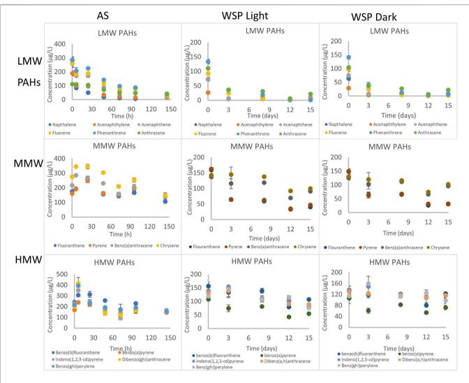
FIGURE 2 | Disappearance of PAHs under aerobic conditions with activated sludge and facultative inocula (under light and dark conditions). Concentration determined in the combined phase (dissolved and particulate). AS refers to activated sludge, WSP refers to waste stabilization ponds. LMW, MMW and HMW refers to low molecular weight, middle molecular weight and high molecular weight respectively.
