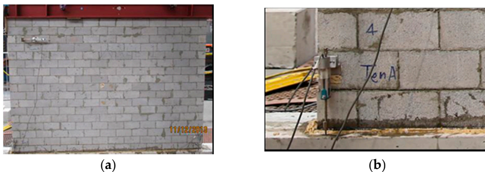
Figure 8. In-plane shear wall testing of TLM masonry walls [72]: (a) in-plane shear testing arrangement and (b) sliding failure of a TLM wall.
