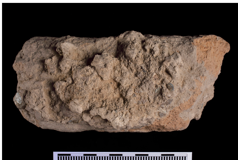
Fig. 5: Mudbrick bearing traces of mud mortar (93.545.294.1). The coarse aggregate of the mortar, rich in micaceous and calcium carbonate aggregate, is visible on the vertical interstice of the brick (N. Gail; © Gygaia Projects).
