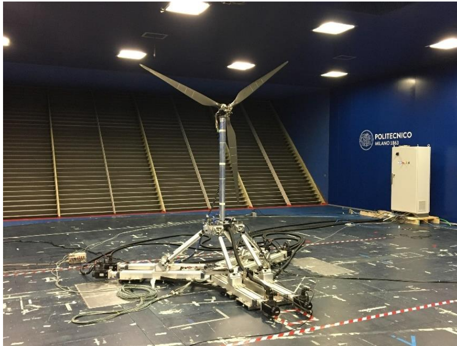
Fig. 2 – Representative example of a wind tunnel, i.e. GVPM facility [46], with a wind turbine model tested by means of HIL technique.
