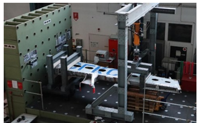
Figure 5. Airbus A320 wing installed on a loading floor at Empa, Switzerland.
