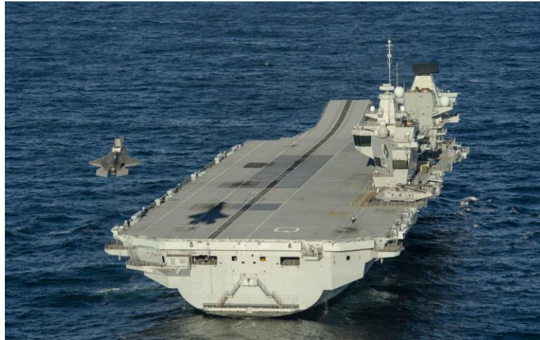
Figure 1-15 F-35B performing an SRVL manoeuvre to the flight deck of HMS Queen Elizabeth © Crown 2019.
