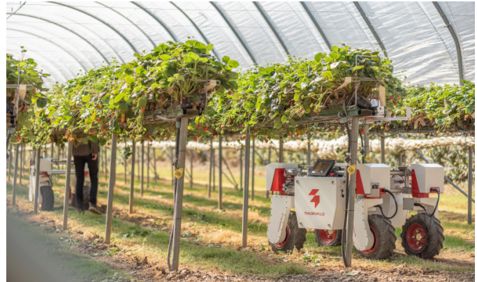
Fig. 1: The Thorvald robot is used for transportation in strawberry production farms.
