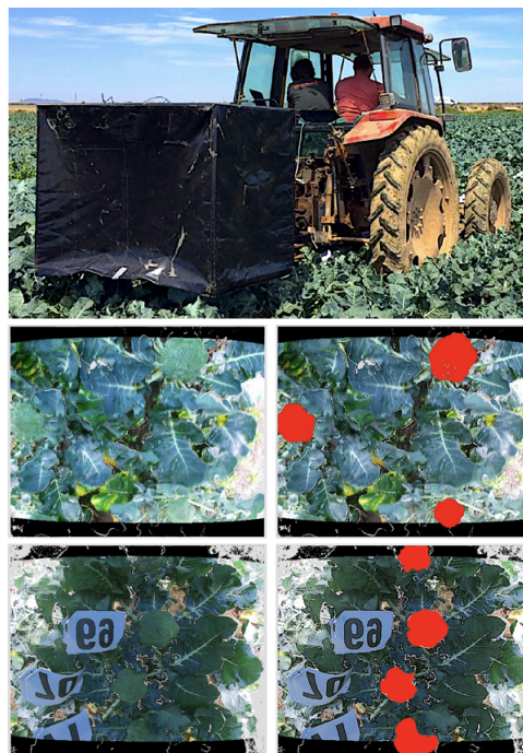
Fig. 2. Shown at the top is the enclosing box mounted at the back of a tractor while collecting data on a broccoli field in Spain. Below are frame samples of the UK dataset (first row) and the Spain dataset (bottom row) collected with this hardware platform. The images on the right column show in red the ground truth annotation on the datasets. The 3D data on the black strips is also processed but no colour texture was matched by the sensor on those regions.
