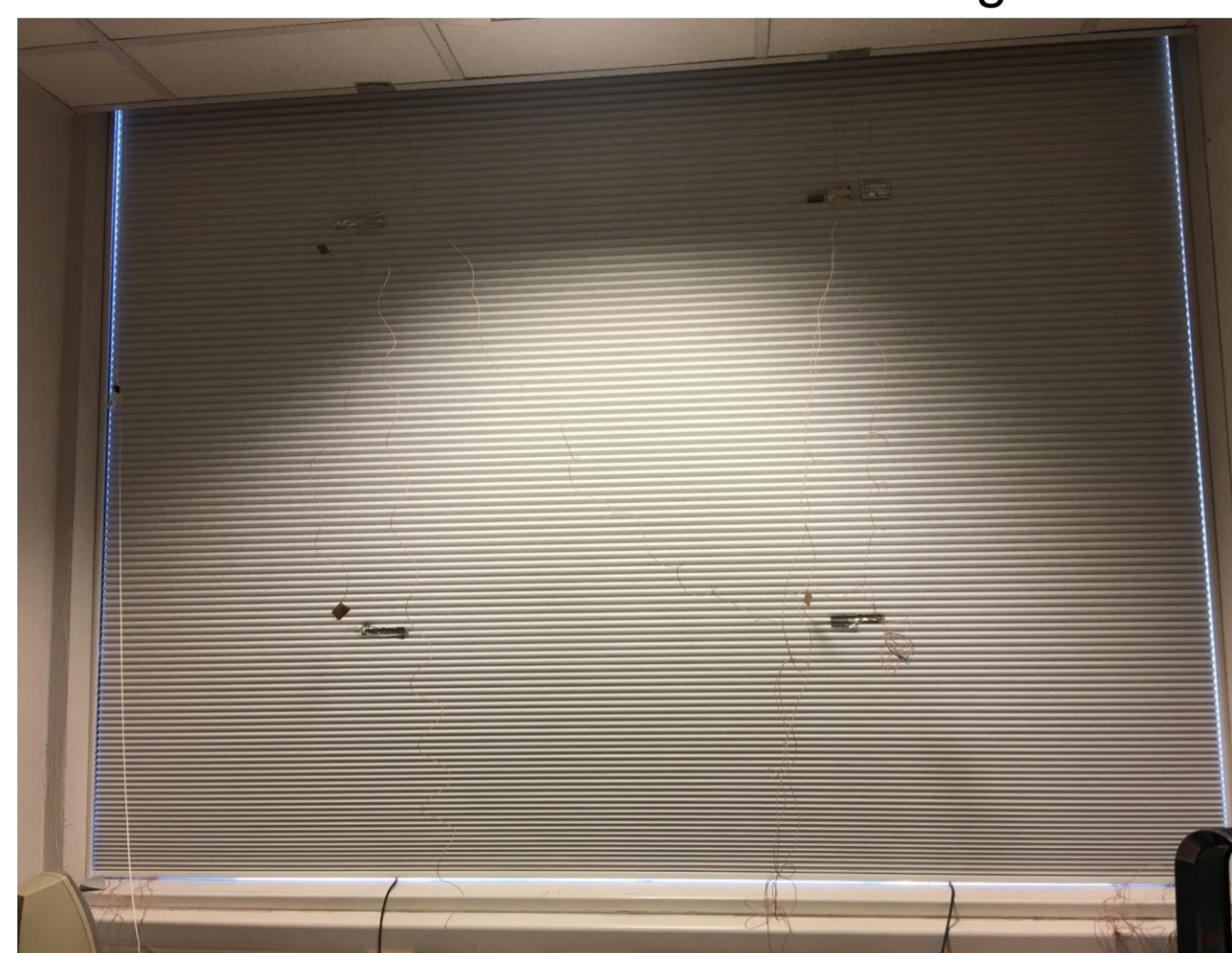
Figure 3: Thermocouples attached to the blind
