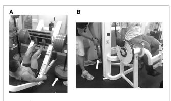
**FIGURE 2** | Training equipment to allow accentuated eccentric loading. Inclined leg press with weight-releasers (A) and manually loaded/unloaded weight plates on the knee extension device (B).
