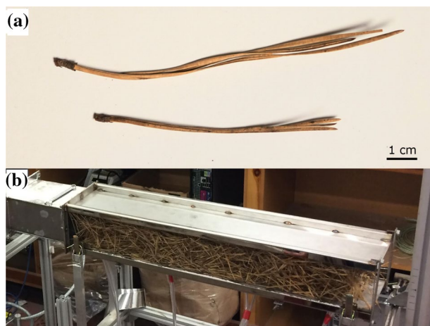
Fig. 2 a Example of Pinus rigida needles, which are grouped with three individual needles on one fascicle. b Example of fuel bed packing for the pressure drop experiments
