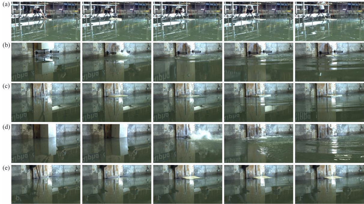
Fig. 6. Image series of experiments conducted at h = 1.00 m: (a) mechanism A, (b) B, (c) C, (d) D and (e) E. The shown examples of mechanisms A, B and E were conducted with the 0.800 \text{ m} \times 0.500 \text{ m} \times 0.250 \text{ m} block (type 2) and the examples of mechanisms C and D with the 0.800 \text{ m} \times 0.500 \text{ m} \times 0.500 \text{ m} block (type 1). The time intervals between the images are 2.67 \text{ s} for (a) and (e) and 1.33 \text{ s} for (b) to (d).
