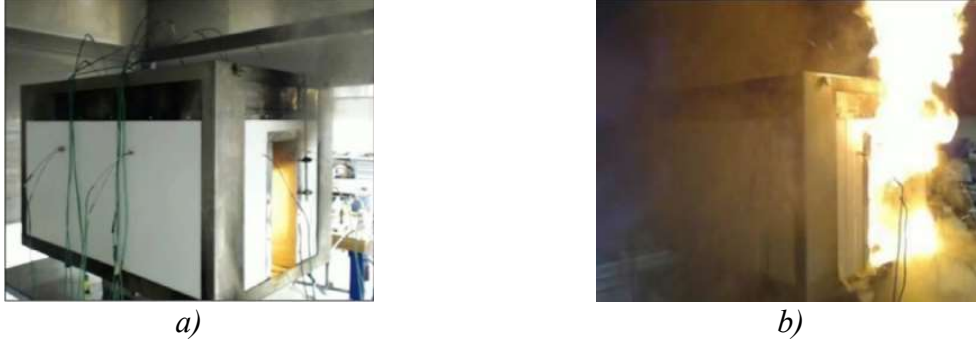
Figure 4: a) 1/5 scale experiment resulting in no-flashover. b) 1/5 scale experiment resulting in flashover. Reused with permission from Leisted 15 .
