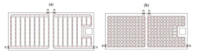
**Figure 17.** (a) Harp-channel absorber plate; (b) grid-channel absorber plate (reprinted from [101], with permission from publisher).
