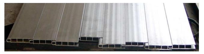
Figure 8. Assembly of aluminium finned flow channels (reprinted from [75], with permission from publisher).
