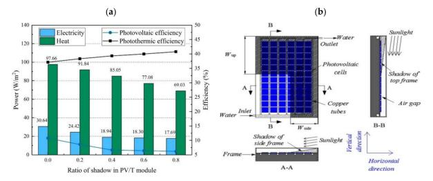
**Figure 20.** (a) Change in electrical and thermal efficiency as a function of shadow ratio; (b) frame shadow on PV/T collector surface (reprinted from [114], with permission from publisher).
