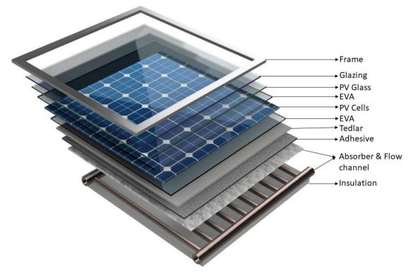
Figure 7. Detailed parts of typical water-based PVT collector.
