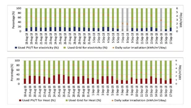
**Figure 14.** Percentage of PVT contribution to supply the electrical and heat demands for 31 days (reprinted from [93], with permission from publisher).
