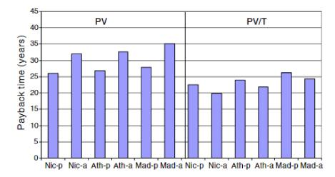
**Figure 33.** Payback times of conventional PV and hybrid PVT system for three different locations (Ni— Nicosia, Ath—Athens, Mad—Madison) and two PV technologies (p—polycrystalline, a—amorphous) (reprinted from [72], with permission from publisher).
