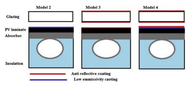
Figure 18. Different configurations of PVT plate (reprinted from [108], with permission from publisher).
