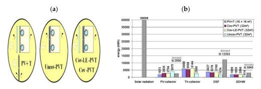
**Figure 9.** (a) Four different configurations; (b) annual energy performance for four configurations (reprinted from [76], with permission from publisher).
