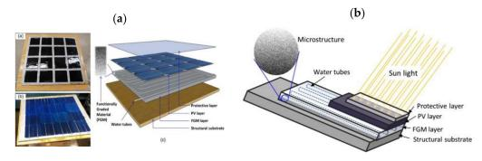
**Figure 27.** (**a**) Hybrid PVT FGM schematic—first design; (**b**) layers of BIPVT—second design (reprinted from [126], with permission from publisher).
