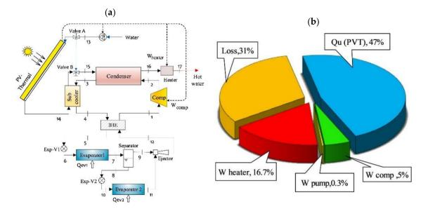
**Figure 13.** (a) Schematic of the system; (b) distribution of energy incident on PVT from the Sun at irradiation =  $945 \text{ Wm}^{-2}$  and water mass flow rate = 0.013 kg/s (reprinted from [92], with permission from publisher).
