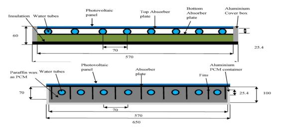
Figure 22. PVT-water and PVT-PCM-water configurations (reprinted from [116], with permission from publisher).
