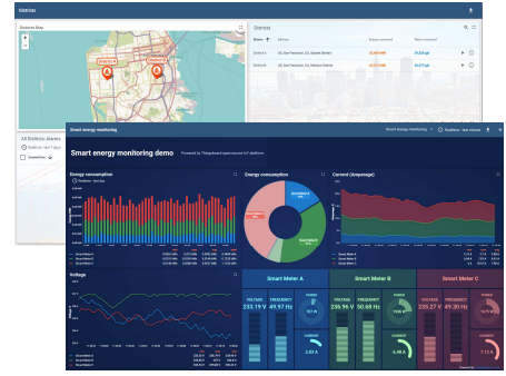
Fig. 2 Developed web-based dashboard using the Thingsboard IoT platform.
