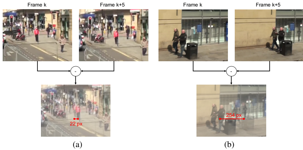
Figure 4.10: Samples from MOT17-13 showing the effect on the image plane when the camera undergoes a dominant (a) translation motion and (b) rotation motion. Note that the person in red in (a) moves 22 pixels as the camera just perform a translation while the person in black in (b) moves 254 pixels, more than an order of magnitude of difference for the same temporal difference and similar depth to the object. Frames k and k + 5 are chosen for the sake of clarity in the example. Source images from [125].
