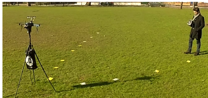
Figure 4.17: Experimental setup. A loudspeaker is carried by a person who walks in front of the drone that is placed on a tripod. The noiseless sector is indicated with yellow marks on the ground.
