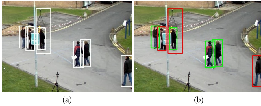
Figure 4.4: Example of strong and weak detections at frame 43 (crop) in PETS09-S2L1. (a) Fused detections \mathbb{Z}_k ; (b) strong (green) \mathbb{Z}_k^+ and weak (red) \mathbb{Z}_k^- detections after classification. Source images from [94].
