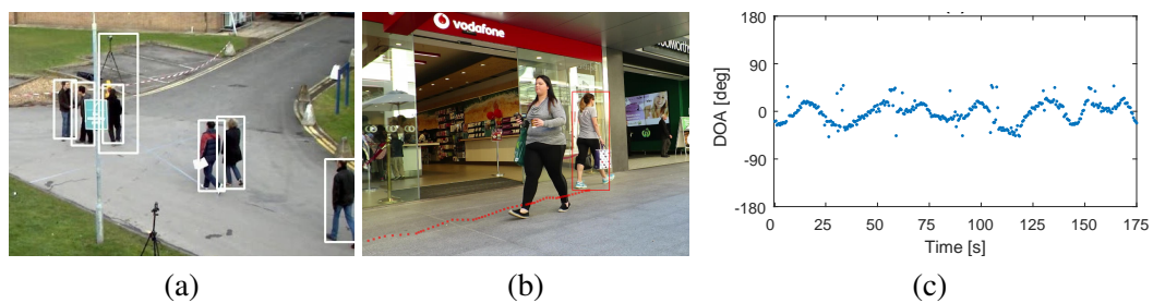
Figure 1.2: Sample of the three types of observations considered in this thesis. When the sensor is a camera: (a) bounding box and (b) point; and, when the sensor is a microphone array, (c) direction of arrival (DOA). Note that the bounding box in (b) is just shown for visualising that the observed points indicate the location in between a person's feet. Images (a) and (b) from [125].
