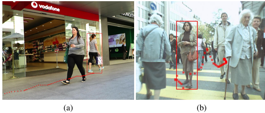
Figure 2.1: Moving pedestrians recorded from (a) static camera and (b) moving camera. Both pedestrians are following a (similar) linear trajectory in the real world but the apparent motion on the image planes is not linear when the camera moves. The bounding box indicates the location of the person in the current time instant. Red solid squares indicate the location of the object in each time instance in the last 2 seconds. Source images from [94].
