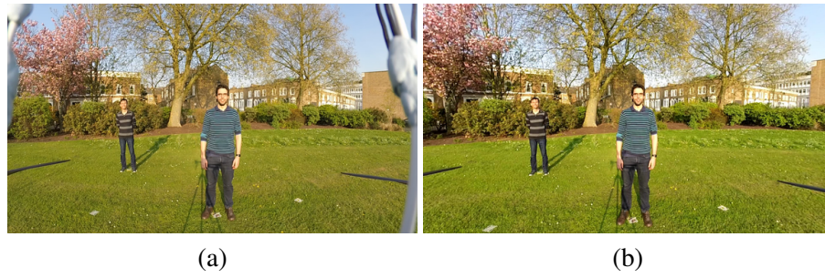
Figure 3.1: Image captured by the camera mounted on the drone (a) before and (b) after image undistortion.
