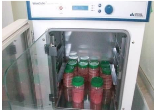
Fig-2: Preparation the Specimens for porosity test and saving it in the incubator
