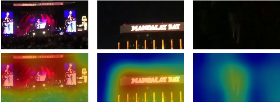
Figure 5.3: Examples of the attention weighting on arbitrary video frames: sampled video frames from the same video (top), attention maps of the corresponding frames (bottom). Red colour indicates high attention weights, whereas blue indicates low ones.
