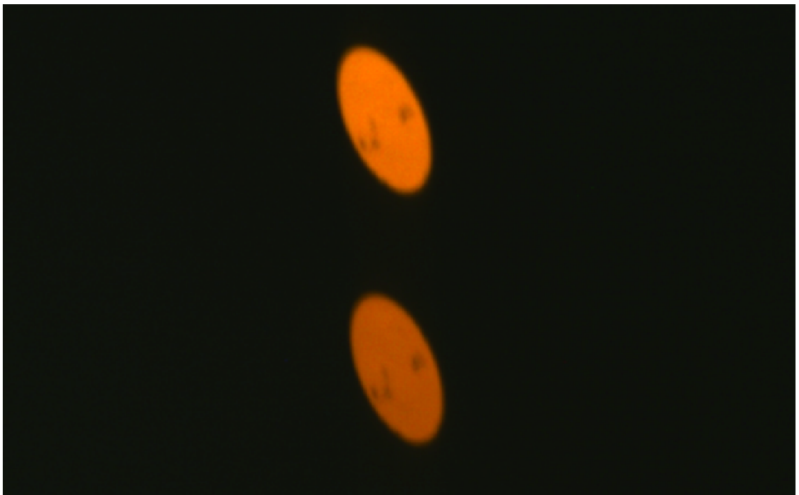
Figure 2.11: Image of the Sodium D-doublet spectrum produced by an early prototype of the QMSPEC instrument. Each of the resolution elements are a monochromatic image of the optical fibre head which feeds the instrument. The effect of Beta-anamorphism is clear with the circular fibre head imaged as a tilted and elongated ellipse.
