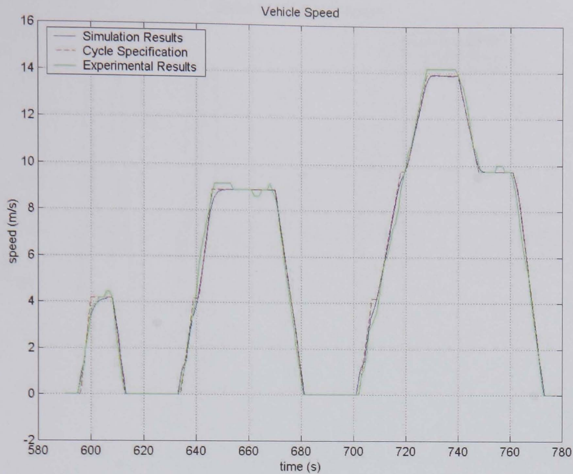
Figure 52 – Simulation v Experimental Vehicle Speed During One Section of the NEDC
