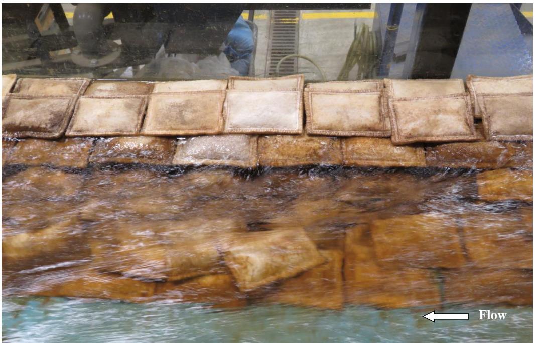
(b) The slump of upper layer bags on the bottom layer
