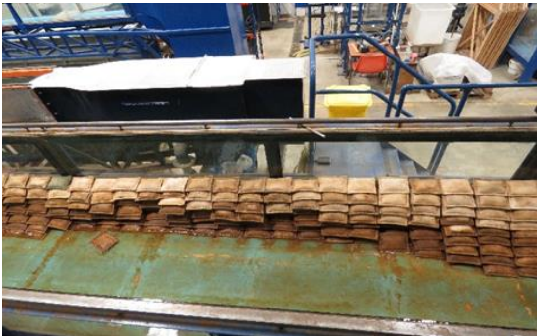
(c) Failure zone (slide zone) after high-water depth condition test
