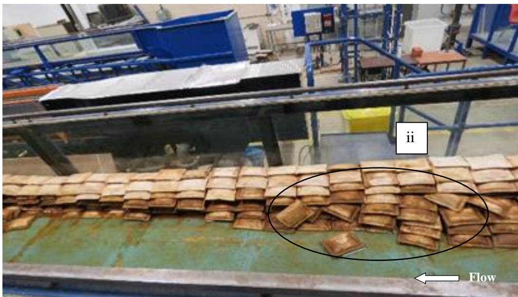
(b) Complete failure: sliding and pullout geobags
