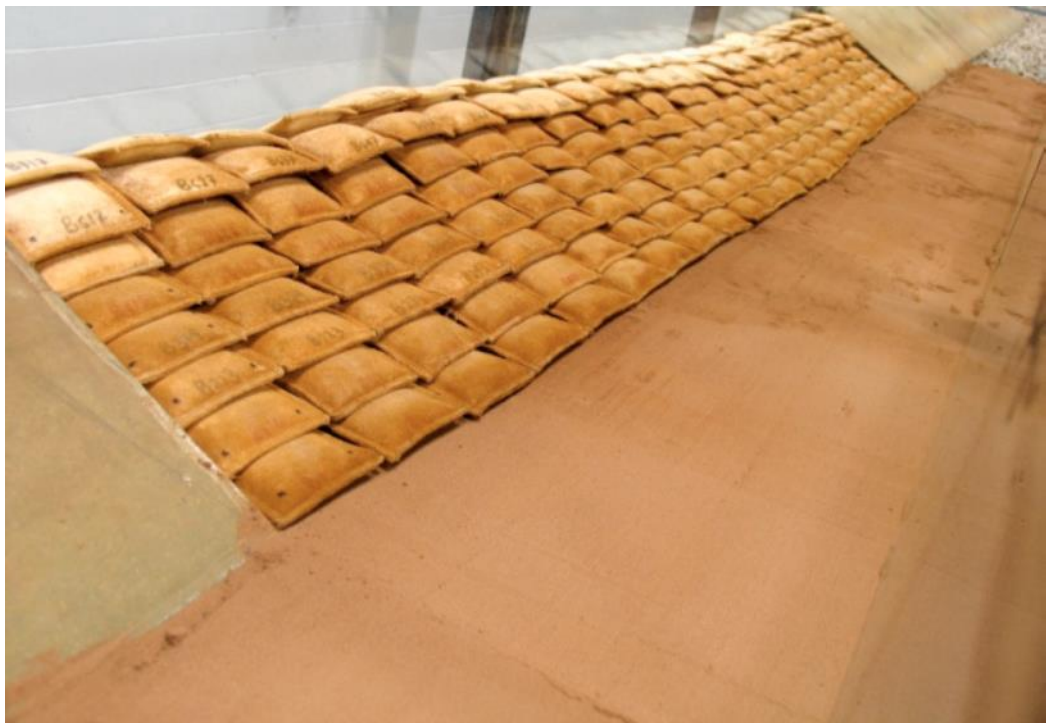
(A2) Geobag revetment on the sandbed
