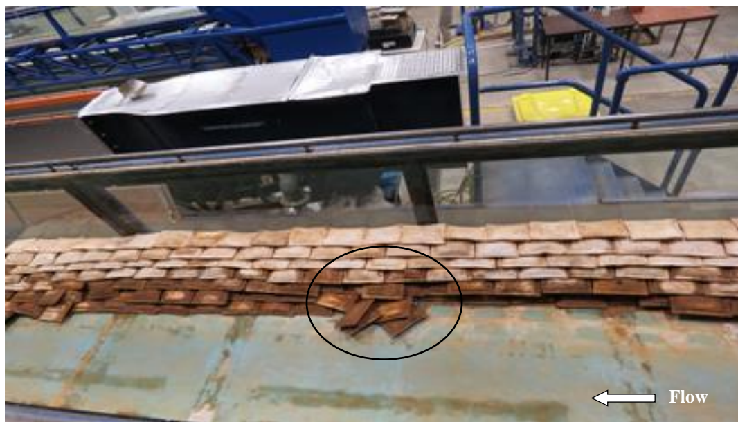
(b) A clump of collapsed bags
