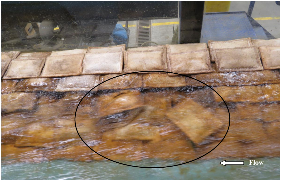
(a) initial displacement due to pullout, partial uplifting and turbulent bursting
