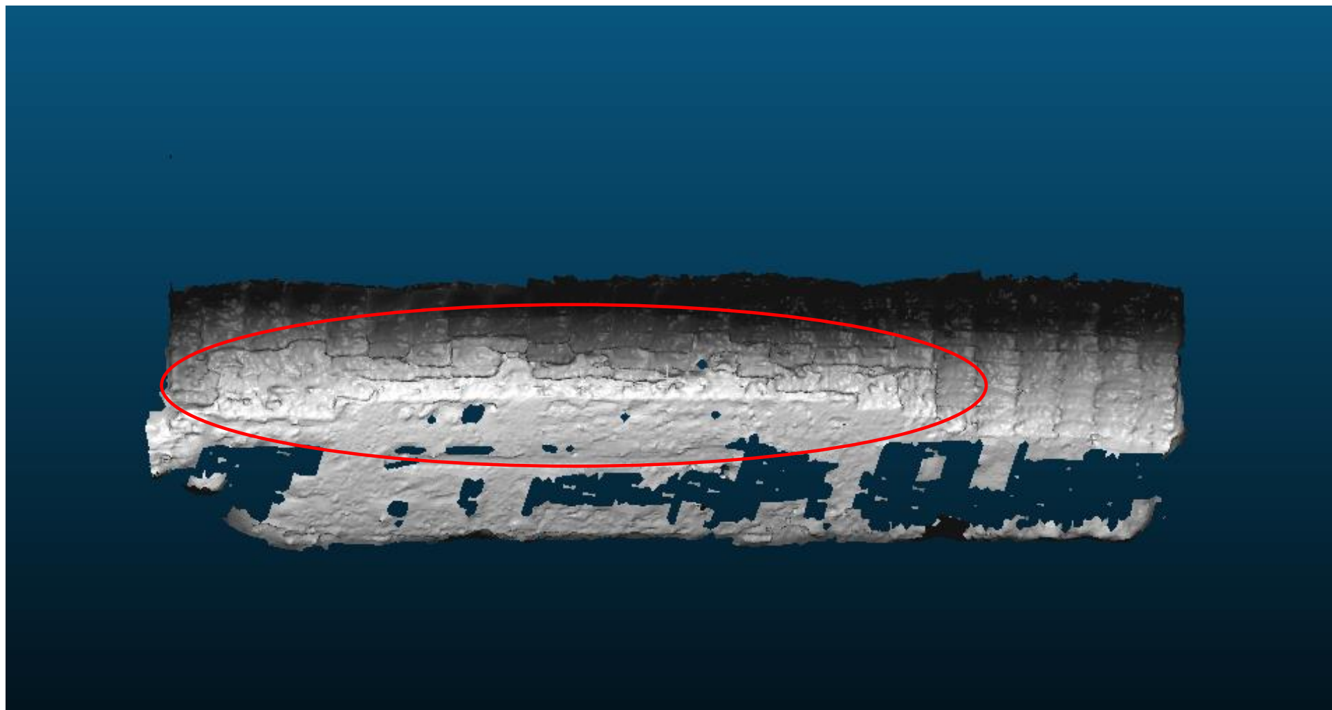
Figure 4.24 (c): Failure zones for 1V:1.25H side slope.
