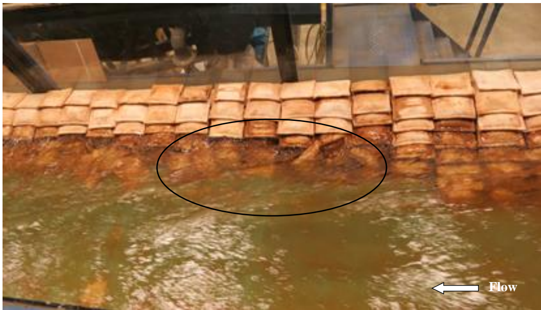
(a) Turbulent bursting–induced flow through revetment voids and sliding
