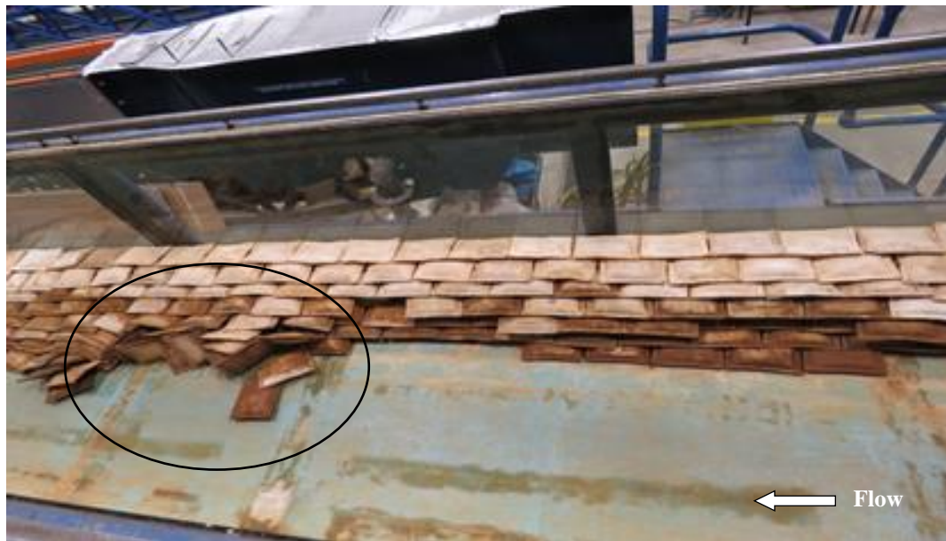
(b) Failure Zone: pullout and dislodging
