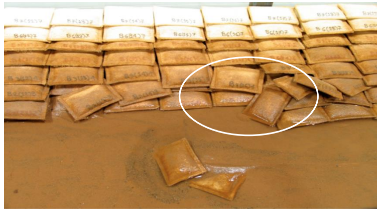
(A1) End of the experiment showing failure mostly involved the bottom-most layer.
