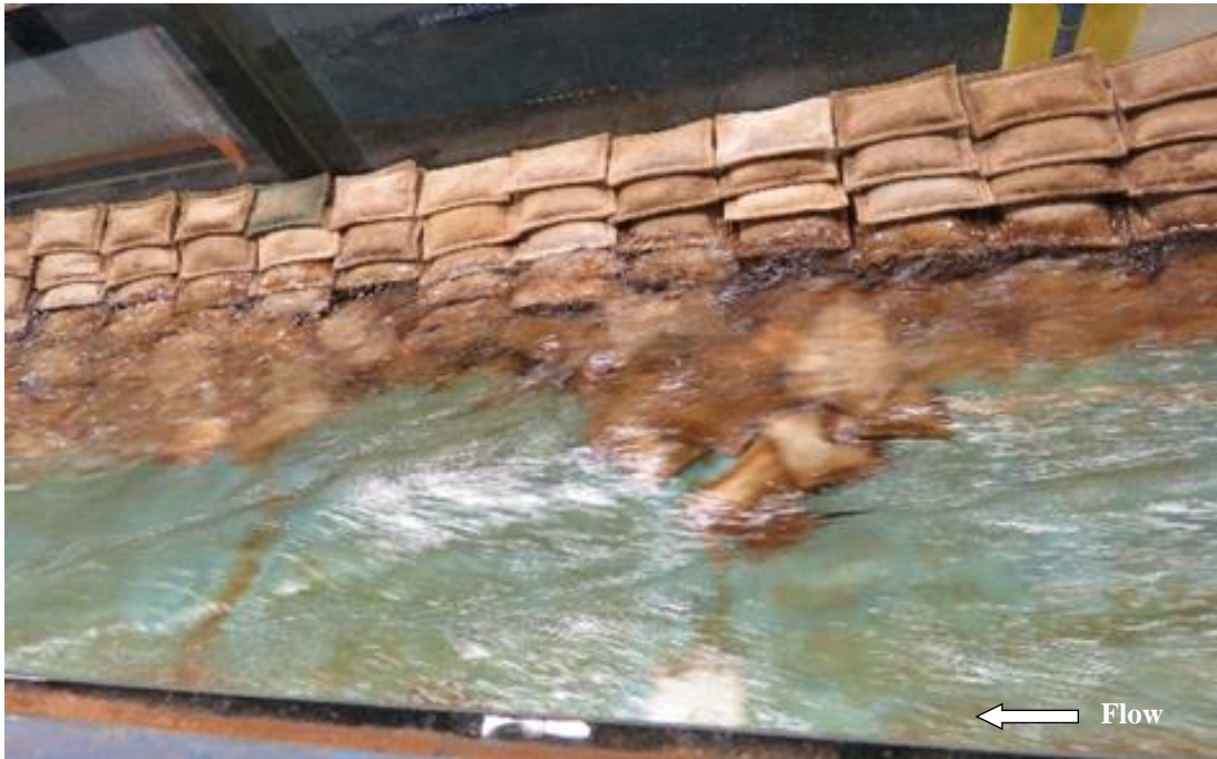
(b) Magnitude of the revetment failure at the beginning of the test due to vertical sliding, high water level
