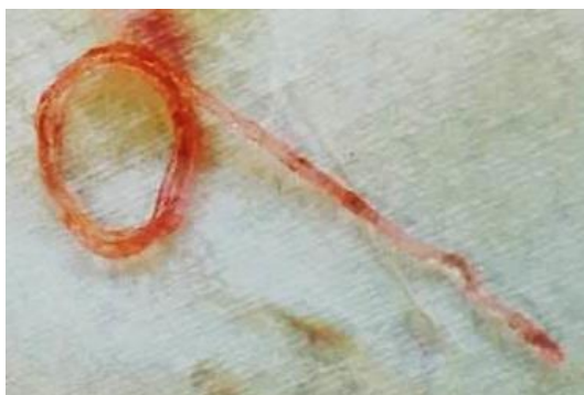
Figure 5.18 – Coaxially extruded structure released from 0.8% w/v gelatine support bath
