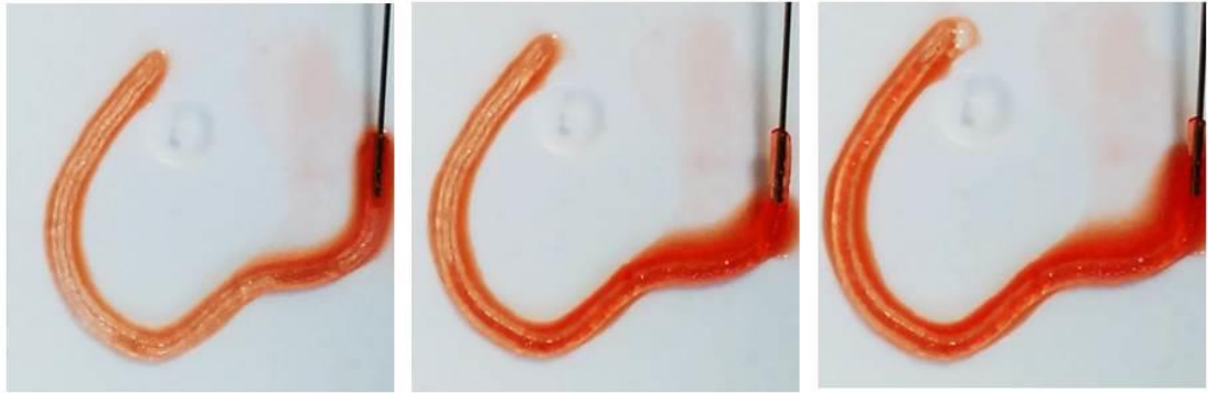
Figure 5.16 – Cut section of coaxially extruded filament is perfused with red dye solution to show successful internal channel formation
