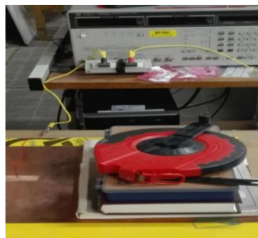
Figure 146: Rough capacitor formed by a square-roughness-model and copper plate connected to the HP4921
