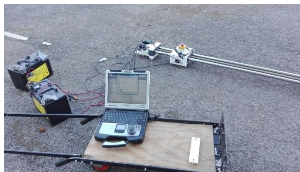
Figure 111: Height distribution measurement of an area of degraded pavement behind the Gisbert Kapp building using a laser profiling instrument
