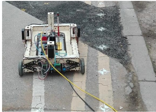
Figure 18: Robotic platform carrying the capacitive-coupled resistivity system on the pavement behind the old library at the University of Birmingham
