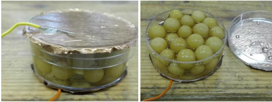
Figure 161: Test rig including epoxy fillers surrounded by water
