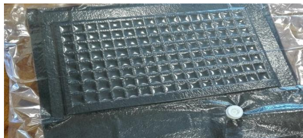
Figure 144: Acrylic squared, perforated sheet placed on the soft foam inside a vacuum bag and used to model a rough surface layer
