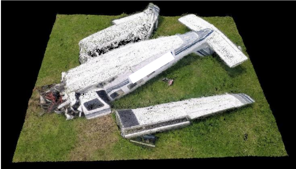
Figure 3.4: Point cloud reconstruction from sUAV scan
