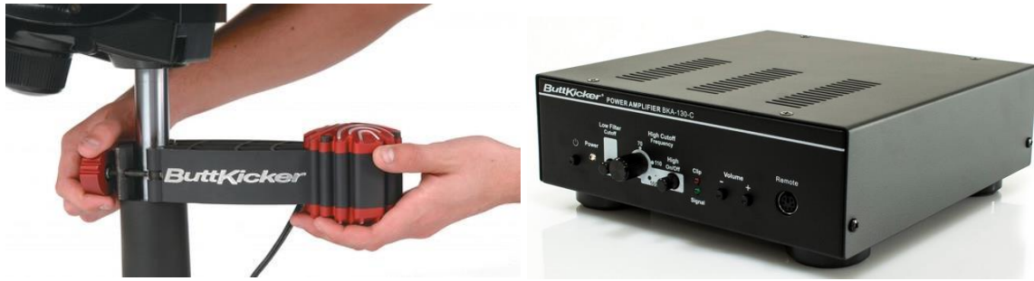
Figure 6.1: Buttkicker Gamer2 Vibration device mounted on chair stem (Buttkicker, 2017)
