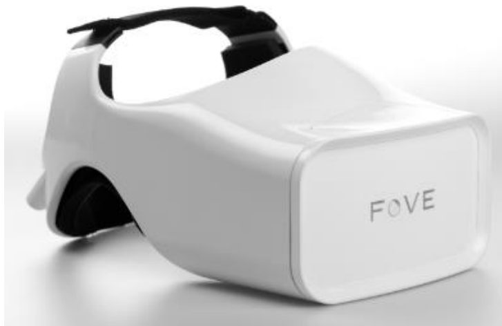
Figure 6.2: FOVE HMD with integrated eye-tracking sensors (FOVE, 2017)
