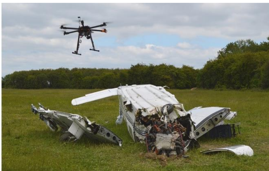
Figure 3.3: sUAV performing photogrammetry scan
