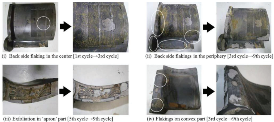
Fig.4. Damage to specimens, observed in the experiment.
