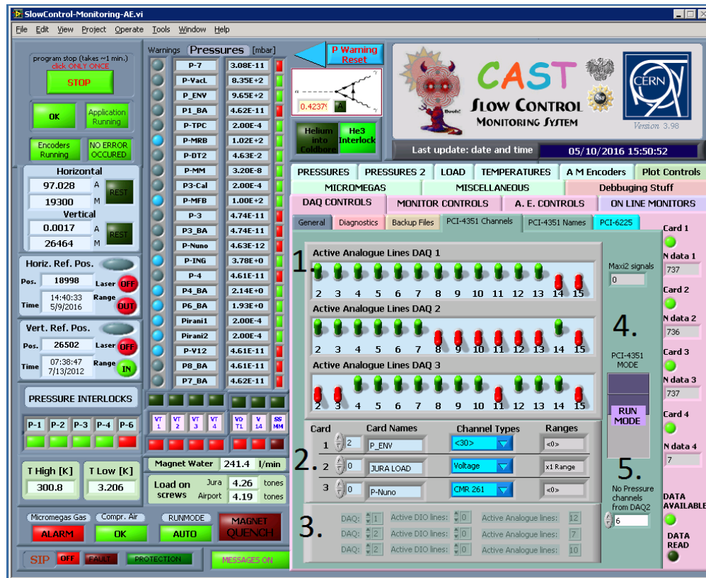
FIGURE 3.13: The active channels of the analogue cards DAQ 1-3
