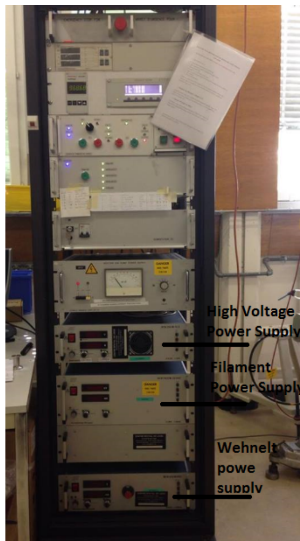
FIGURE 4.5: The power supplies of the X-ray beam line.
