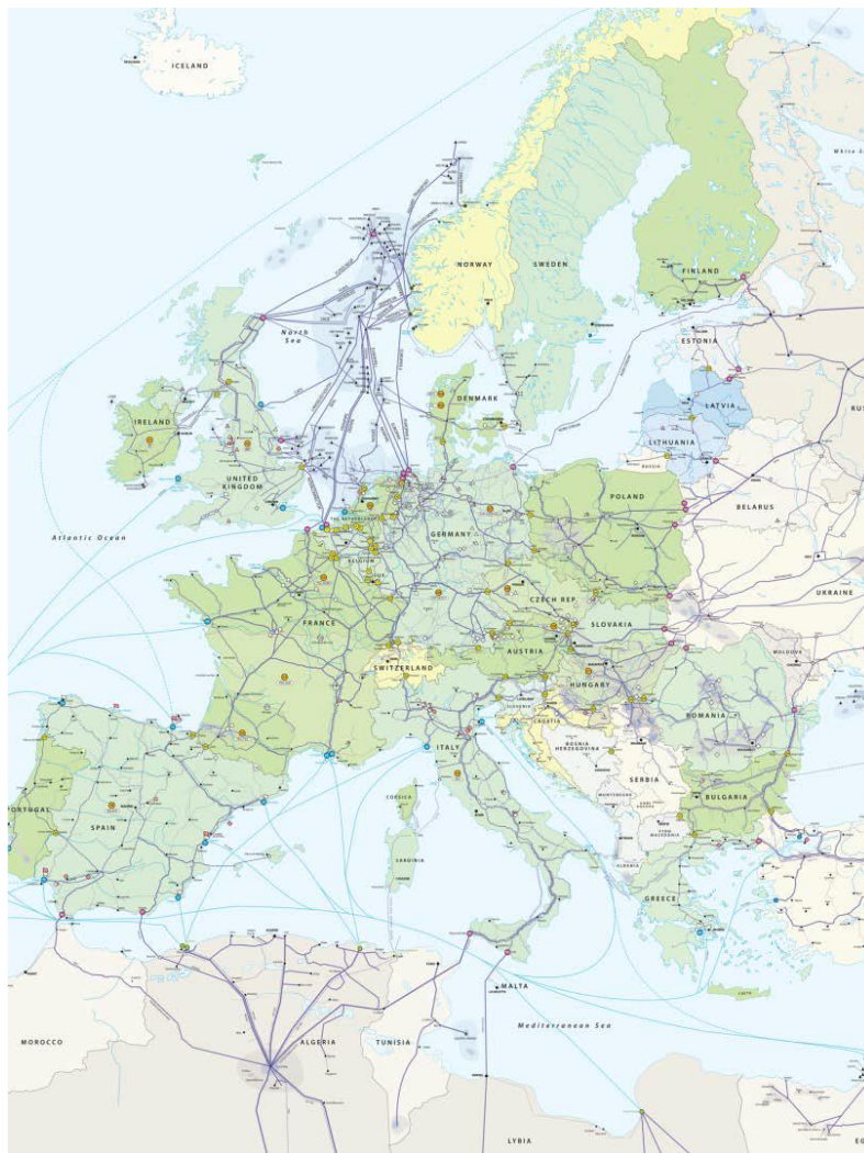
Fig. 2. 11 Existing and planned onshore and offshore pipelines in Europe and North Africa.
