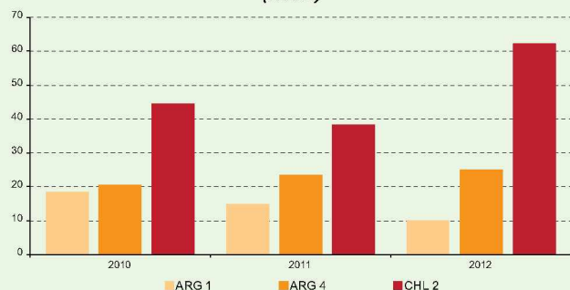
Figure 7 ELECTRICITY CONSUMPTION PER OPERATING HOUR OF A SHIP-TO-SHORE CRANE (kWh)
