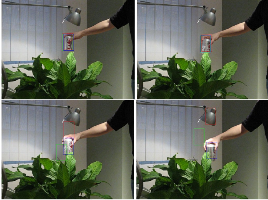
Figure 6.13: Tracking sequence: Frame 5, 13, 21, and 34 are shown (starting from the top left one in clockwise direction). Red box is for SIR-PF, Green box is for bat algorithm and Blue box is for the proposed algorithm for Table. 6.4
