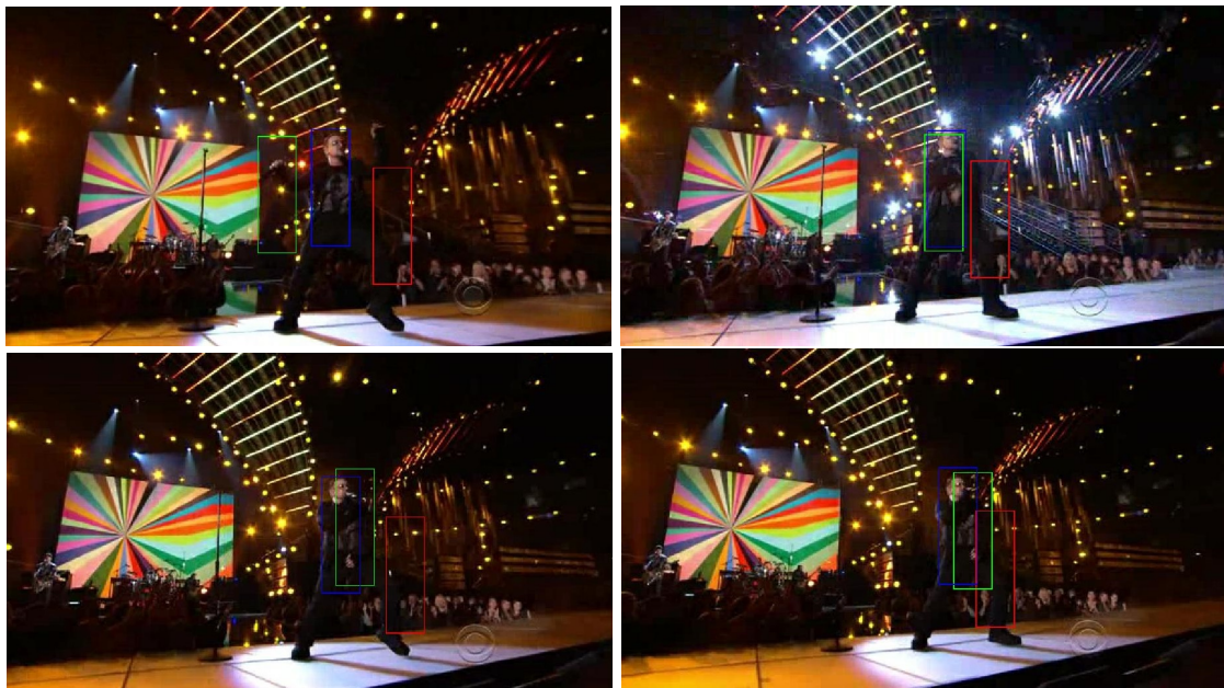
Figure 6.26: Tracking sequence: Frame 28, 36, 43, and 48 are shown (starting from the top left one in clockwise direction). Red box is for SIR-PF, Green box is for bat algorithm and Blue box is for the proposed algorithm for Table. 6.7
