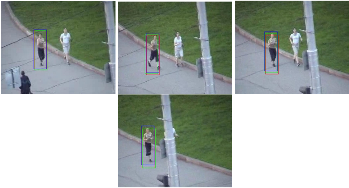
Figure 6.21: Tracking sequence: Frame 3, 26, 38, and 55 are shown (starting from the top left one in clockwise direction). Red box is for SIR-PF, Green box is for bat algorithm and Blue box is for the proposed algorithm for Table. 6.6
