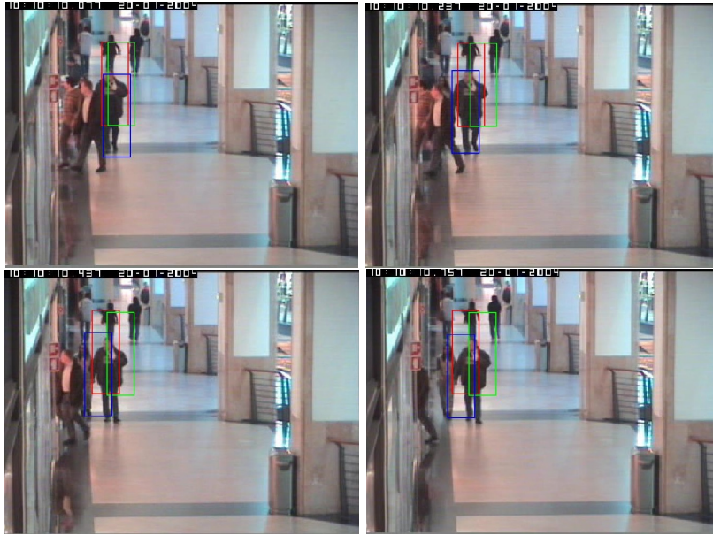
Figure 6.35: Tracking sequence: Frame 252, 256, 262, and 269 are shown (starting from the top left one in clockwise direction). Red box is for SIR-PF, Green box is for bat algorithm and Blue box is for the proposed algorithm for Table. 6.9
