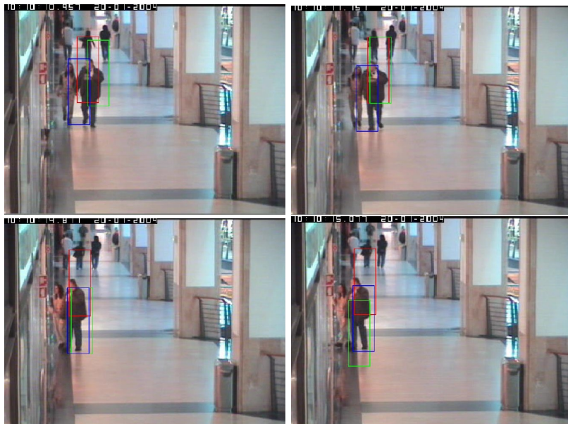
Figure 6.36: Tracking sequence: Frame 275, 294, 373, and 377 are shown (starting from the top left one in clockwise direction). Red box is for SIR-PF, Green box is for bat algorithm and Blue box is for the proposed algorithm for Table. 6.9
