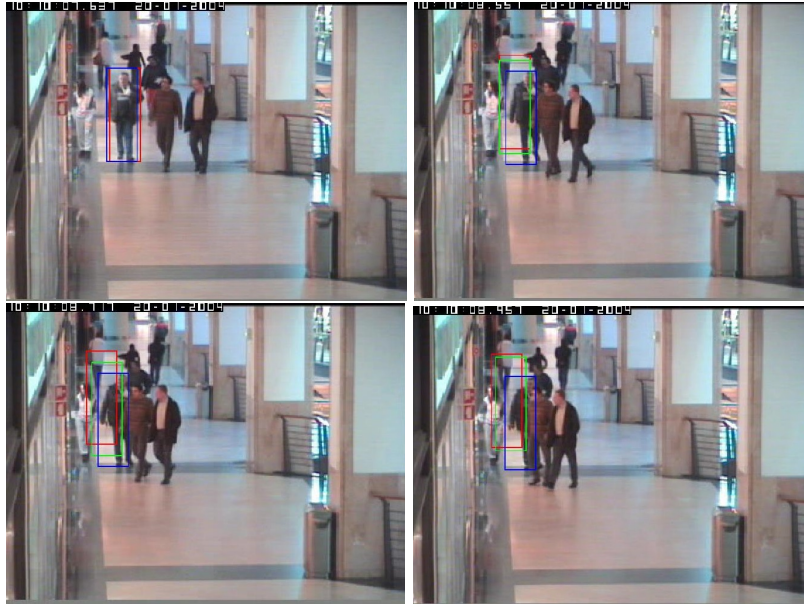
Figure 6.33: Tracking sequence: Frame 192, 214, 218, and 224 are shown (starting from the top left one in clockwise direction). Red box is for SIR-PF, Green box is for bat algorithm and Blue box is for the proposed algorithm for Table. 6.9
