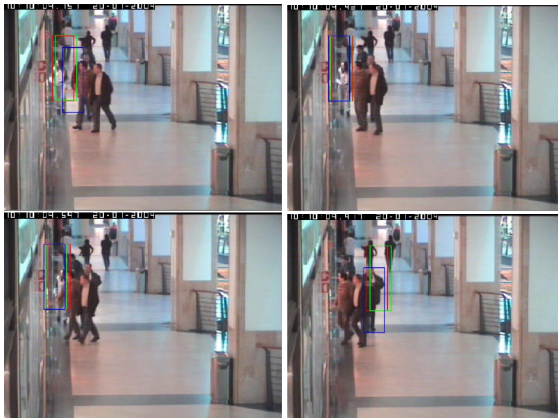
Figure 6.34: Tracking sequence: Frame 229, 237, 240, and 248 are shown (starting from the top left one in clockwise direction). Red box is for SIR-PF, Green box is for bat algorithm and Blue box is for the proposed algorithm for Table. 6.9
