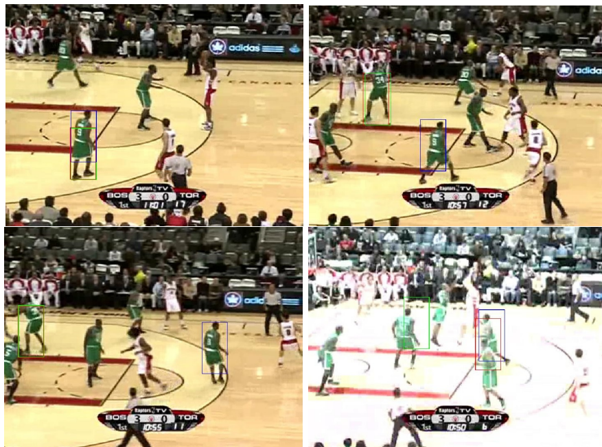
Figure 6.3: Tracking sequence: Frame 334, 460, 506, and 651 are shown (starting from the top left one in clockwise direction). Red box is for SIR-PF, Green box is for bat algorithm and Blue box is for the proposed algorithm for Table. 6.1
