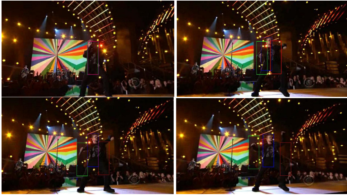
Figure 6.25: Tracking sequence: Frame 7, 20, 23, and 27 are shown (starting from the top left one in clockwise direction). Red box is for SIR-PF, Green box is for bat algorithm and Blue box is for the proposed algorithm for Table. 6.7
