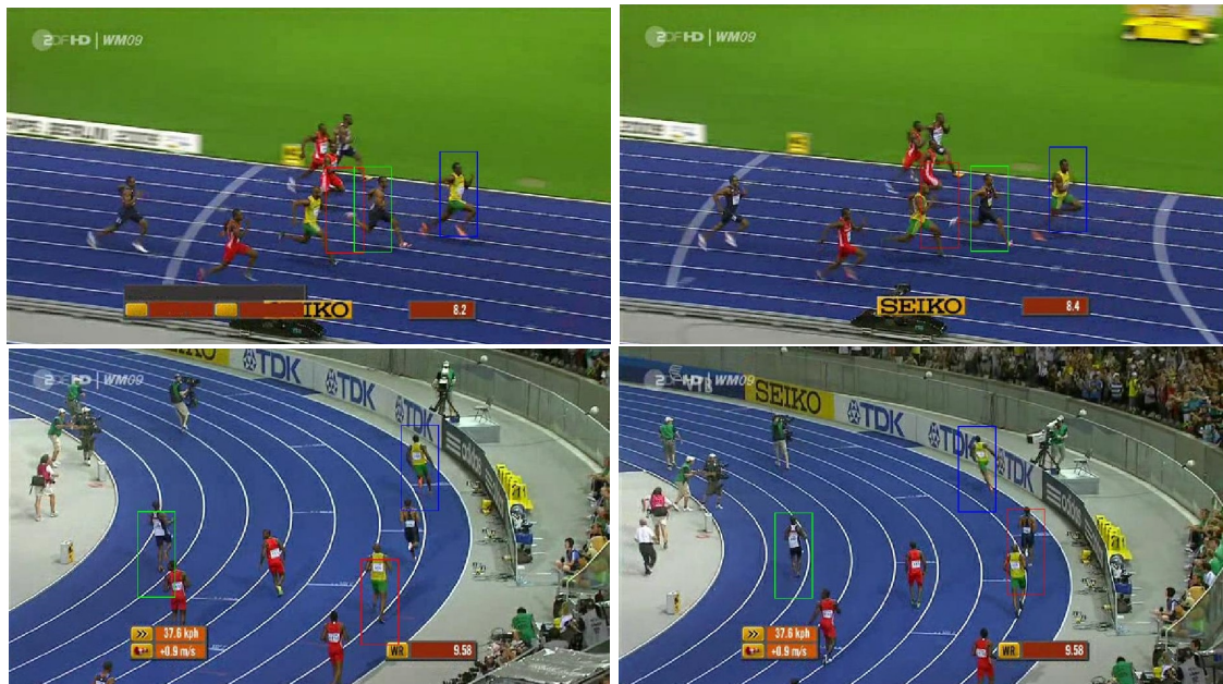
Figure 6.8: Tracking sequence: Frame 195, 200, 330, and 350 are shown (starting from the top left one in clockwise direction). Red box is for SIR-PF, Green box is for bat algorithm and Blue box is for the proposed algorithm for Table. 6.2
