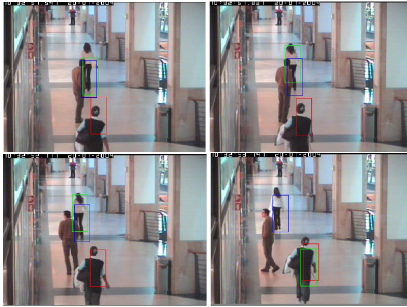
Figure 6.31: Tracking sequence: Frame 485, 491, 513, and 540 are shown (starting from the top left one in clockwise direction). Red box is for SIR-PF, Green box is for bat algorithm and Blue box is for the proposed algorithm for Table. 6.8
