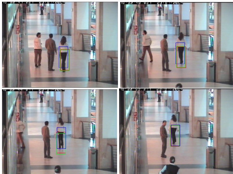
Figure 6.30: Tracking sequence: Frame 376, 419, 428, and 454 are shown (starting from the top left one in clockwise direction). Red box is for SIR-PF, Green box is for bat algorithm and Blue box is for the proposed algorithm for Table. 6.8
