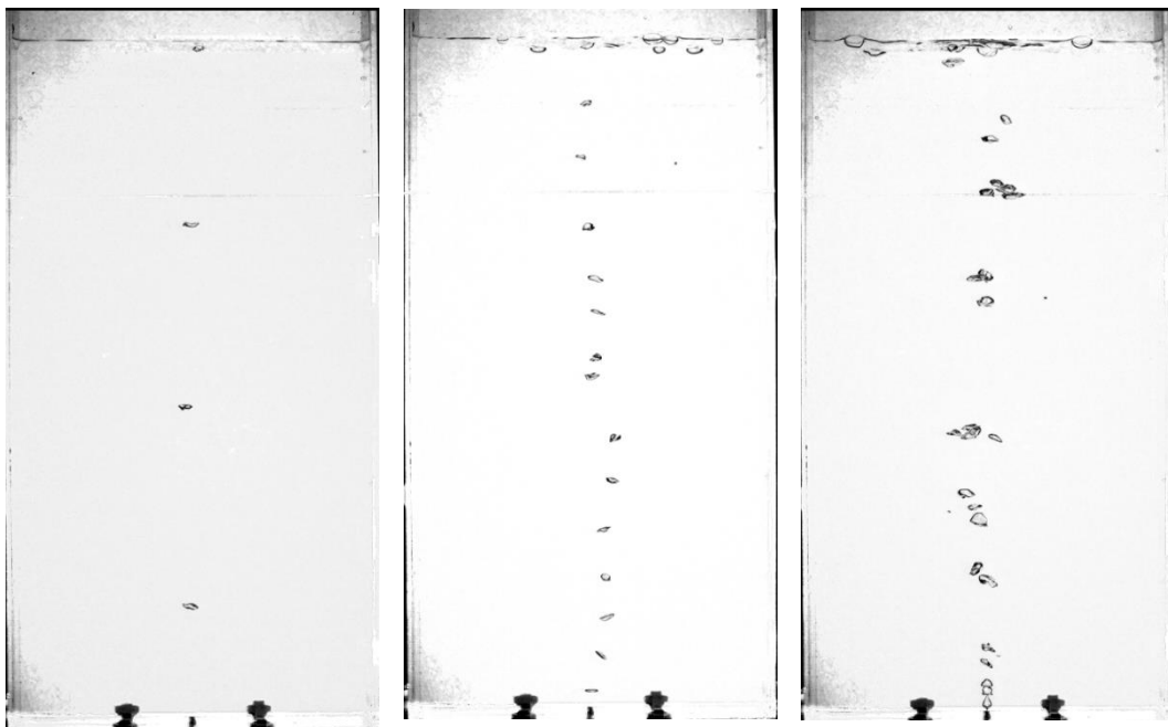
Figure 7 For flow gas rate (a) 10L/h, (b) 20L/h and (c) 30L/h for 0.7 mm diameter nozzle w/o MIBC
