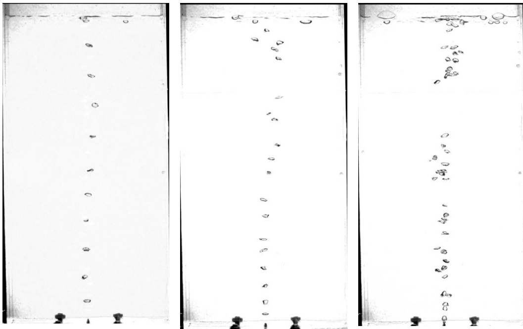
Figure 11 For flow gas rate (a) 10L/h, (b) 20L/h and (c) 30L/h for 0.9 mm diameter nozzle w/o MIBC
