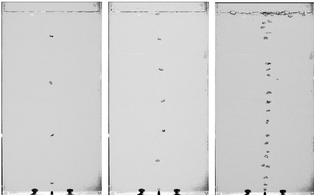
Figure 3 For flow gas rate (a) 10L/h, (b) 20L/h and (c) 30L/h for 0.5 mm diameter nozzle w/o MIBC
