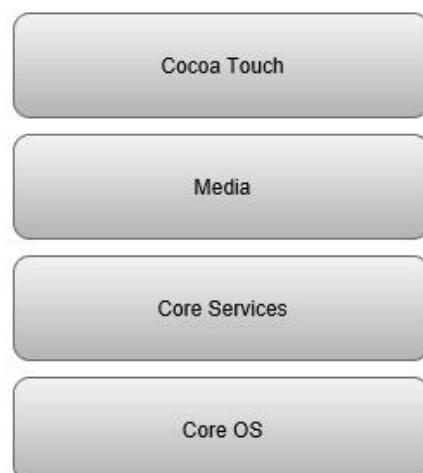
Picture 2. iOS platform architecture, modified from (Apple, 2014).
