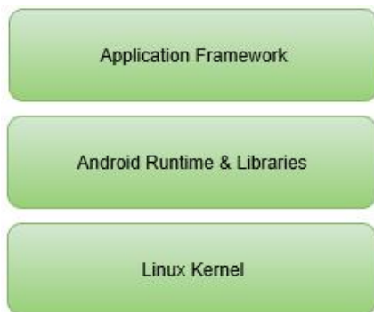
Picture 3. Android platform architecture, modified from (Android Team, 2016).
