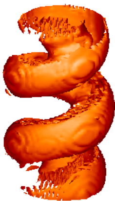
Fig. 6. Isosurface of |j| = 1.2 at t = 30 for the resistive evolution.
