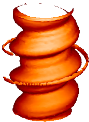
Fig. 8. The isosurface of the current for run 1 with the current concentration seen as a thin thread wrapped around the central current.
