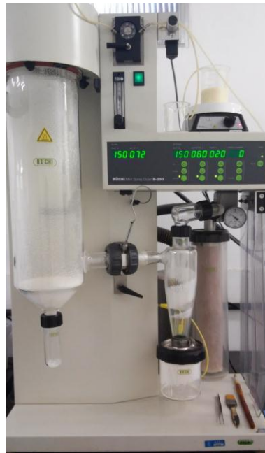
Fig. 1. Spray drying processing
