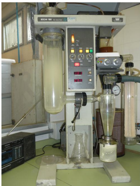
Figure 2. A laboratory spray dryer used to obtain punicalagin in dry form
