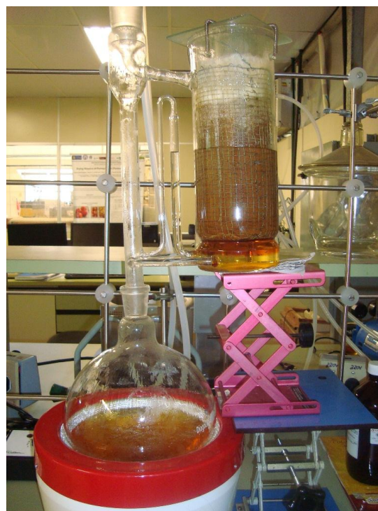
Fig. 1. Extraction process in a Soxhlet equipment
