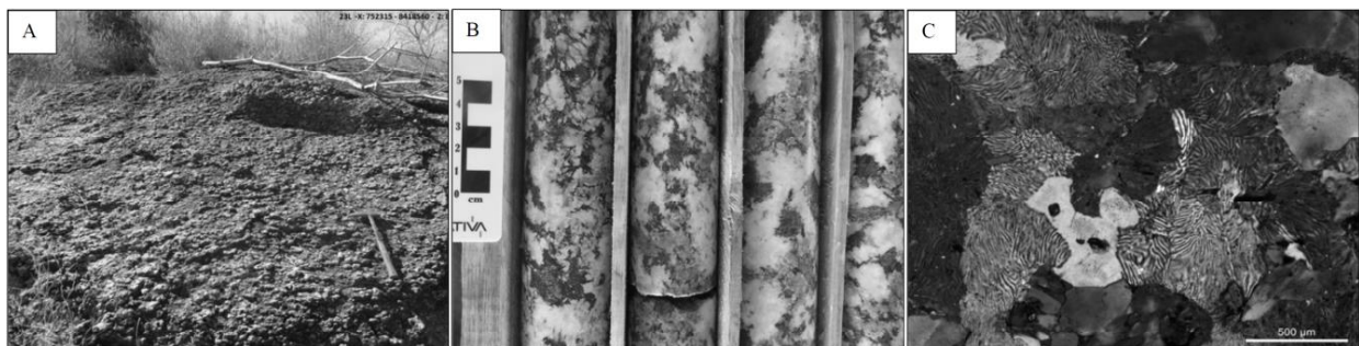
Figure 3. Pictures of the biotite alkali-feldspar syenite from Ceraíma Project. (A) Outcrop, (B) Detail in a sample of borehole, (C) Photomicrography (X nicols) showing the intergrowth of alkali feldspar crystals
