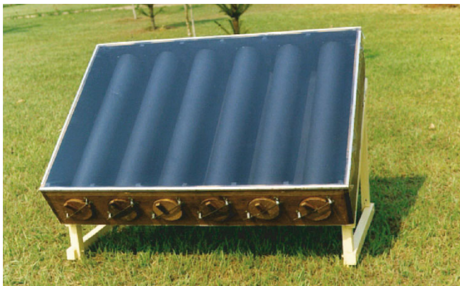
Fig. 1. Solar collector for substrate disinfestations.
