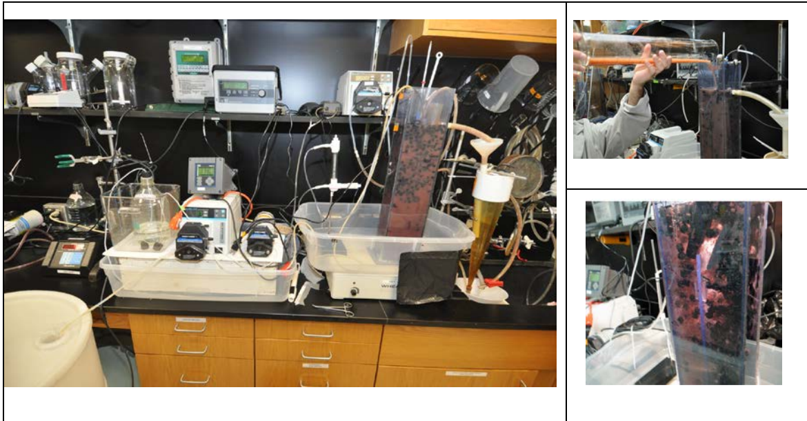
Figure 2: Deammonification treatment using single-tank to perform partial nitrification and anammox in a fluidized continuous flow aerated reactor. A) 5-L reactor set-up, B) Mixing of HPNS with anammox, and C) Reactor detail with plastic carriers inside.
