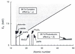
Figure 1. Graphical representation of the dependency of the ratio of Compton and photoelectric effects cross-section on the atomic numbers (Duliu, 1999).
