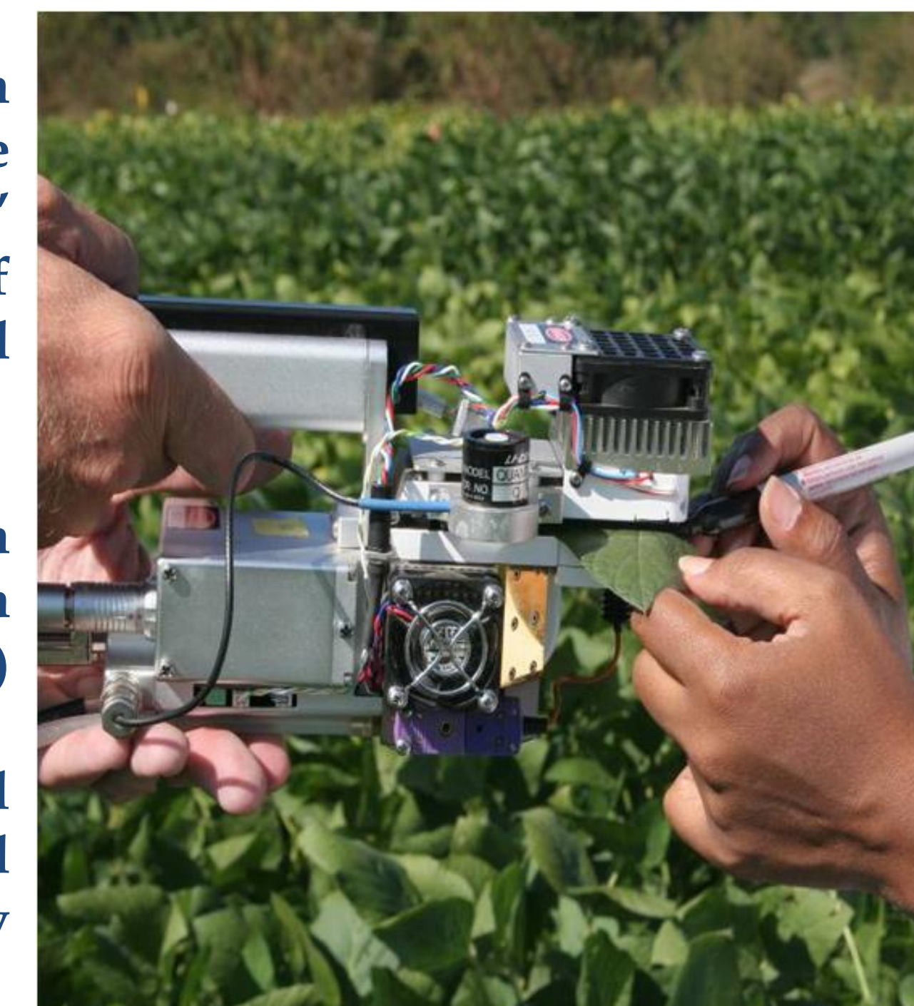
Figure 2: Measurement of net carbon exchange rate using the LI-6400 system under field conditions (Londrina, Brazil) and tagging the location on which measurement was performed with permanent marker.
