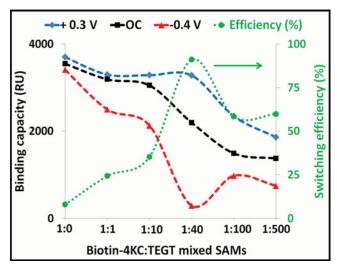
**Figure 2.** The binding capacity under open circuit conditions, an applied positive (+0.3 V) and negative (-0.4 V) potential as well as switching efficiency of the biotin-4KC:TEGT mixed SAMs at solution ratios of 1:0, 1:1, 1:10, 1:40, 1:100 and 1:500.
