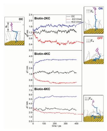
**Figure 4.** The conformational changes of biotin-2KC, biotin-4KC and biotin-6KC under different electric fields, along with the MD simulation snapshots. The black arrows show the directions of the applied electric fields. Water molecules and hydrogen atoms are omitted for clarity. *d* is defined as the gap distance variation between the biotin and TEGT matrix.
