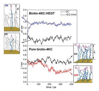
**Figure 5.** The conformational changes of biotin-4KC:HEGT (up) and pure biotin-4KC (down) under different electric fields, along with the MD simulation snapshots. L is defined as the gap distance variation between the biotin and gold surface.
