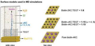
**Scheme 2.** The surface models used in the MD simulations. The purple, blue and dark green parts of the biotin-nKC chain represent the biotin motif, lysine and cysteine residues, respectively. The orange dots, light green balls, yellow balls and short grey chains denote water molecules, chloride ions, gold atoms and TEGT, respectively.
