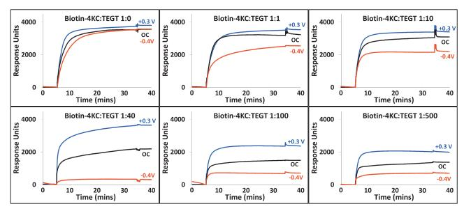
Figure 1. SPR sensorgram traces showing the binding of neutravidin (37 μg.mL<sup>-1</sup>) to the biotin-4KC:TEGT mixed SAMs at solution ratios of 1:0, 1:1, 1:10, 1:40, 1:100 and 1:500 under open circuit conditions (no applied potential), an applied positive (+0.3 V) and negative (-0.4 V) potential.
